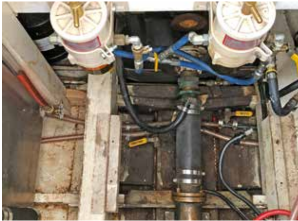
dual Racors and dripless serviced
