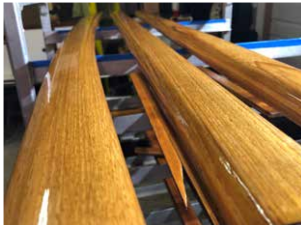
hand rails removed, stripped, and 10 coats Epifanes
