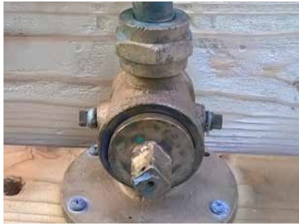
all thru-hulls removed, lapped, and greased
