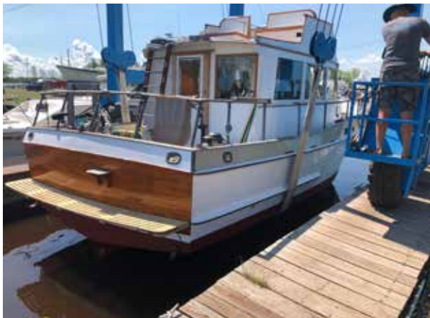
bottom received 3 coats Interlux Micron CSC
