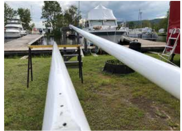
mast and boom stripped , primed and 4 coats Brighside
