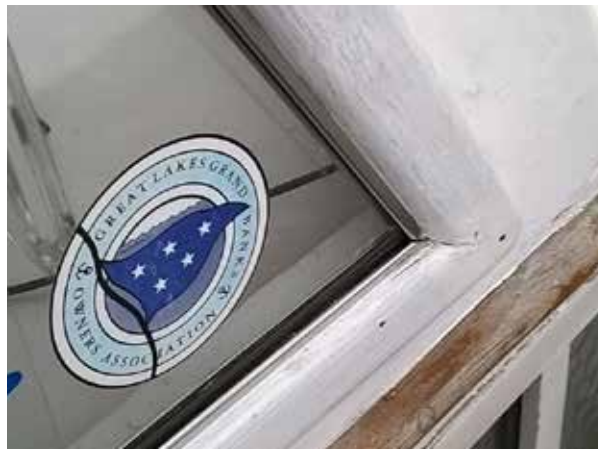
all sliding windows removed and new channel installed
