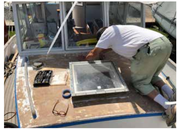
hatch removed and 10 coats of Epifanes
