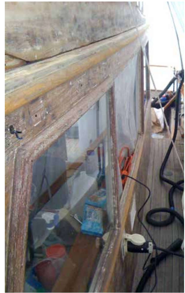
exterior stripped to bare, CPES coated
