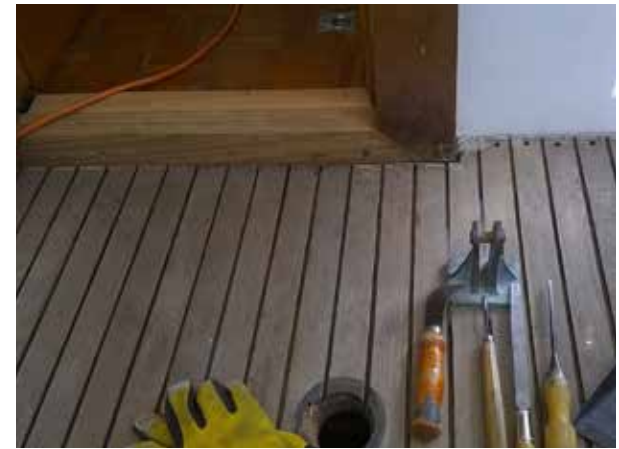
deck seams were cleaned and TDS-440 sealed them
