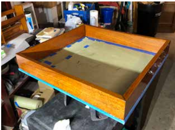
trim able to be removed stripped and 10 Coats Epifanes
